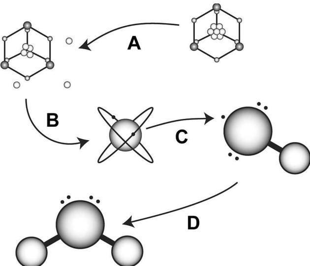
**FIG. 4.** Mechanism of hydroxyl radical with silica hydride. In solution, silica hydride slowly dissociates its embedded hydride anions (A), which interact with the  $1s1s'$  orbital of the hydride anion (B), directly reducing the unpaired electron of the hydroxyl radical (C), water, and  $1s^1$  hydrogen. This mechanism results in no toxic products formed and does not induce a cytotoxic environment.
