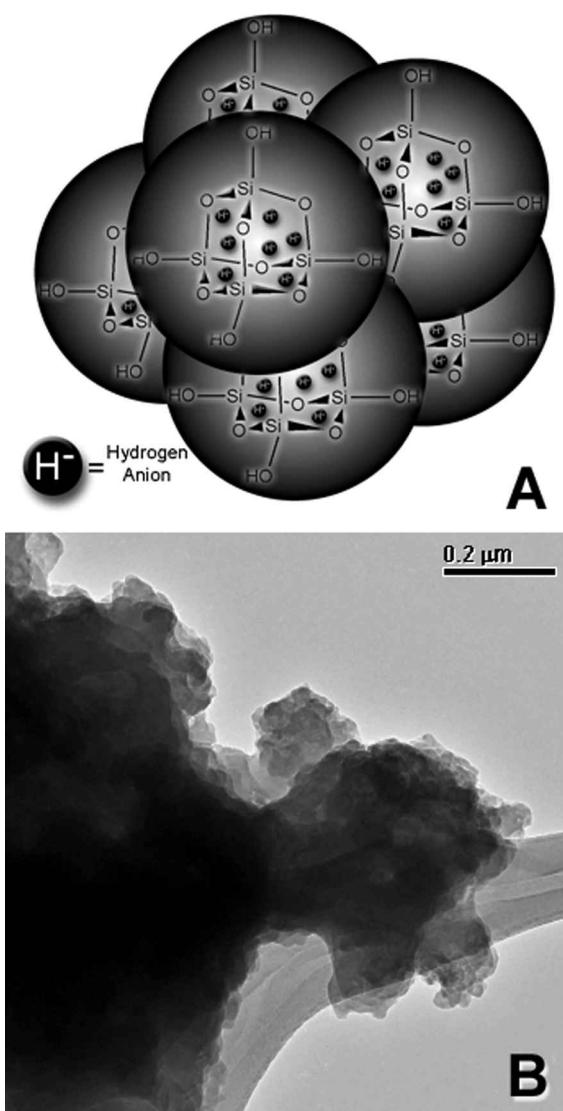
**FIG. 2.** Silica hydride. (A) Graphical model of silica hydride as small, submicron silsesquioxane spheres interstitially embedded with hydride anions. (B) A scanning transmission electron microscopic image of the silica hydride, taken with a Phillips CM30 instrument illustrating the small, spherical constituents of the silica hydride compound.
